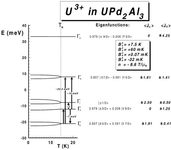
Fig. 1. Energy level scheme of the  $U^{3+}$  ion in  $UPd_2Al_3$ . The arrows indicate transitions that we have attributed to the excitations revealed by inelastic-neutron-scattering experiments [6].
